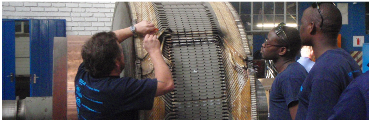
Figure 1: An armature winder and two apprentices 'taking the dope'
